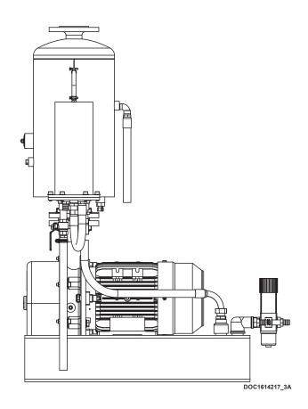
To prevent calcium deposits, use a liquid separator or take necessary measures to prevent calcium in the service liquid.
