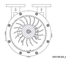
When the pump is started, the liquid ring will rotate at the same speed as the rotor. The rotor is positioned slightly higher than the centre point and divides the liquid ring up into cells. If one were to see the cell in the top position, it would be completely filled with liquid.
