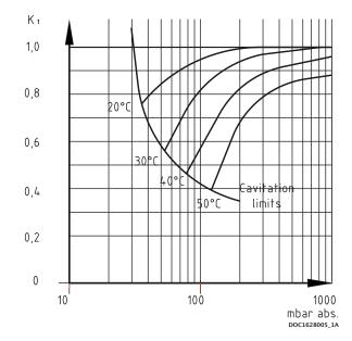
Capacity at service liquid temperature higher than  $15^{\circ}\text{C}$ :
