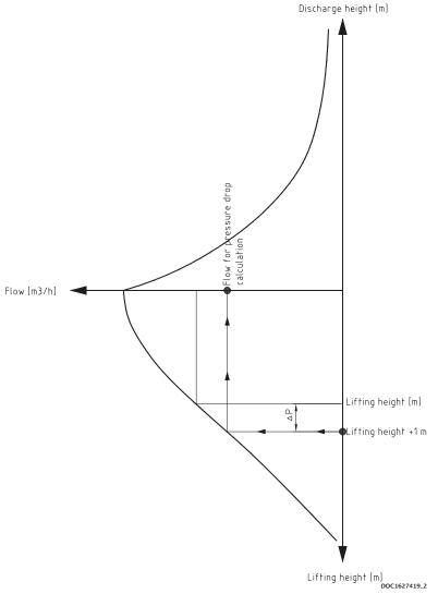
It is possible to calculate the pressure drop manually, but there is a lot of free programs for download. Use the system data to evaluate the pressure drop used as start value. The calculated value can be used to find out if the start value is too low or too high.
