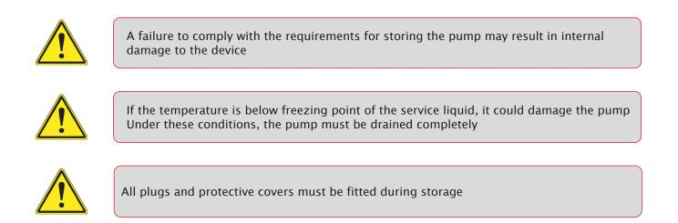
The pump's service liquid is drained on delivery, and the pump can be immediately stored in accordance with the technical specifications.
