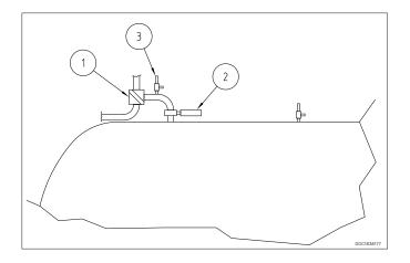
Please ensure the installation of a safety valve in both the pipe system and the tank. The safety valve in the pipe system should be designed to maintain pressure at safe levels when the pump operates at full speed. The safety valve in the tank serves to prevent pressure build-up due to thermal expansion.
